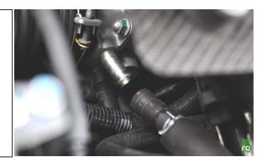
Remove any fasteners that may be installed in the two threaded bosses circled at right.
