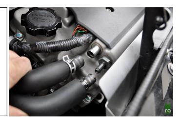
Disconnect the larger PCV hose the same way from the port on the throttle body (shown) and remove the hose from the engine bay.
