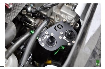
Using oil, lubricate the hose end barbs and force each hose onto the respective hose end (as shown). Next, screw the small 90deg hose (shown) onto the appropriate catch can top fitting. Do not tighten yet. Slide a clamp on and push the hose onto the smaller (PCV valve) barb fitting on the valve cover. NOTE: It might be helpful to loosen the bolts that hold the catch can bracket to the valve cover. This will allow some movement of the catch cans to help get the hoses in place.
