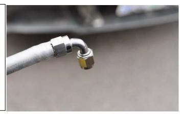
Torque the B-Nut on each hose end to the catch can fittings.
