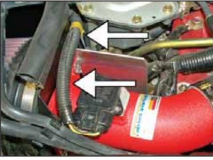
30. Route the mass air sensor electrical connection under the coolant lines and between the heat shield and insulation plate and reconnect the mass air sensor electrical connection as shown.
