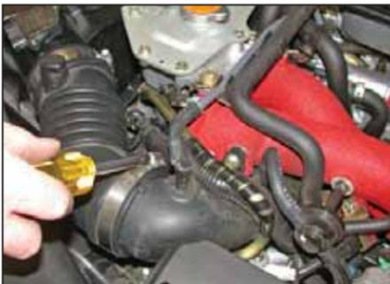
4. Loosen the hose clamp as shown.
