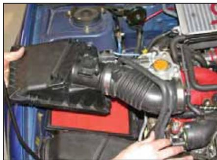
6. Remove the upper air cleaner assembly as shown.
