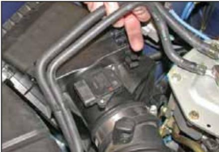
3. Unclip the coolant lines from the top of the air cleaner as shown.
