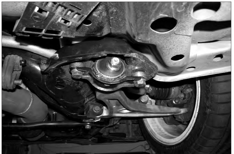
Fig. 3 - Note RHS, offset bushing installed for caster gain.
