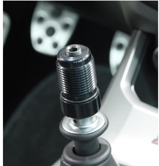
This picture shows outer knob removed from adapter and set screw exposed and ready for adjustment.
