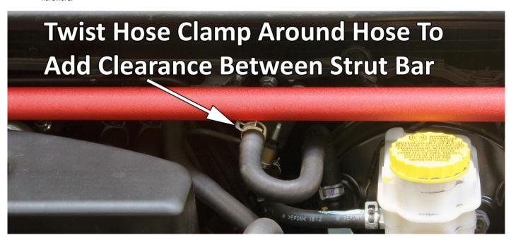
8) Add clearance between strut bar and brake booster hose by either rotating hose clamp down or pushing down on piping to bend it out of the way.
