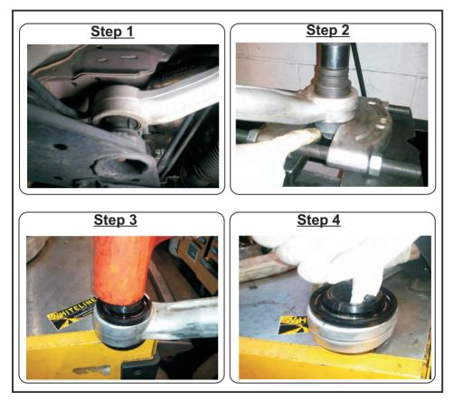
**Step 1:** Raise the vehicle on a lift or alternatively jack the vehicle up and support on jacking stands. Remove the lower splash tray cover and proceed to remove the lower cradle assembly to gain access to the compression rod. Remove the compression rod cotter pin and using a suitable ball joint separating tool press the joint out of the wheel hub assembly.
